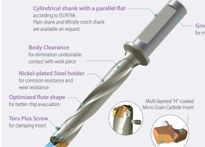
Internal cooling channel for higher drilling performance
